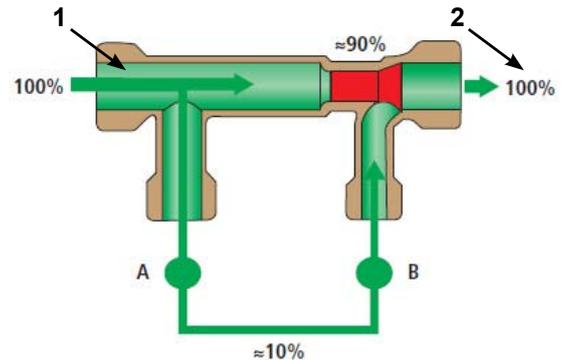
1. The pre-heated water from the WWHRS before it splits to the water heater and the cold inlet of the shower TMV.
