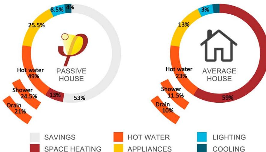
In a Passive House with a similar energy usage profile DHW generation accounts for 48.9% of the overall energy budget. Assuming the showering habits of those in Passive Houses do not differ from the average home, a staggering 20.8% of the energy used in passive houses could be pouring out of the building envelope via the shower drain.
